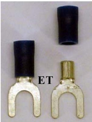
Take four (4) "Spade" Electrical Terminals (ET) #8-10 Stud and remove the plastic sheaths. Insert a piece of 3/32 Rod into the ET's and bend them around the LS as shown.
