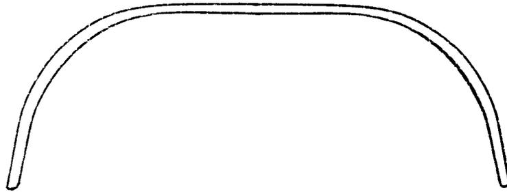
Landing Gear "LG" (2 Req.) 3/32" Rod x 5 1/2" long.
